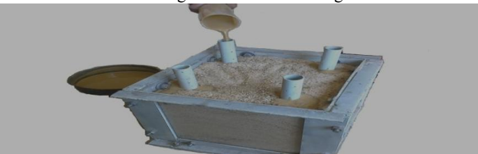
Fig 7.1 Plate load testing of loosest state of sandy soil
