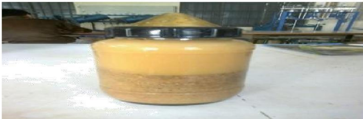
Figure 4.2 Pycnometer test arrangement
