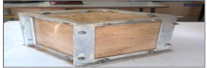
Fig 6.4 shows well grouted sample for certain curing period
